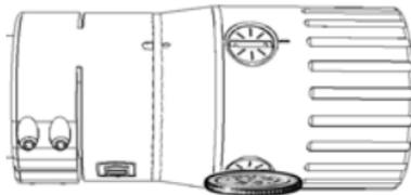
The ScopeX2 utilizes an Adjustment Lock to ensure no loss of zero under recoil. Before adjusting the turrets, remember to loosen this screw with the included 1/16" hex wrench, and to secure this screw when final zero is achieved. Snug this screw lightly with about 5 in/lb of pressure. Do not overtighten.
